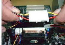
Inserting the second PL-P3/SMP into the processor slot.
